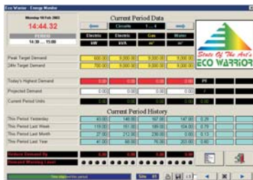
CURRENT HALF HOUR INFORMATION AND PREVIOUS DAY, WEEK, MONTH YEAR CHECK DISPLAYS.
